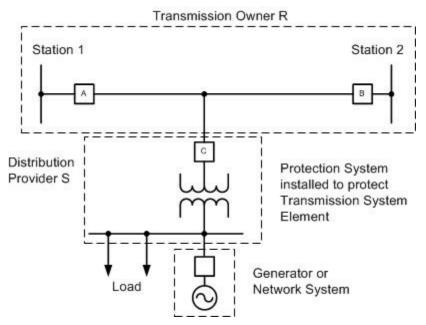
In Figure 3 above, the Interconnected Element between the Transmission Owner and the Distribution Provider is the transmission line or tap between the line and Breaker C.
