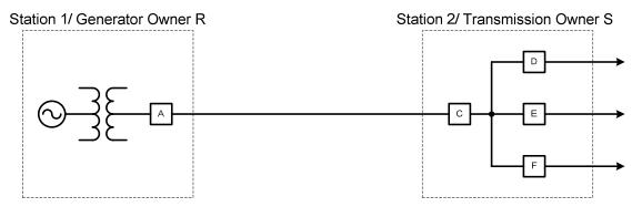
In Figure 2 above, the Interconnected Element between the Transmission Owner and the Generator Owner is the transmission line or bus between Breakers A and C.
