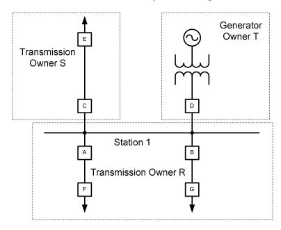
In Figure 5 above, the Interconnected Element between the Transmission Owners R and S and the Generation Owner T is the common Transmission bus. In this example, Transmission Owner S and Generator Owner T are not directly interconnected to each other at Transmission Station 1, and all direct interconnections are between Owner R and each of the other Owners connected to the bus.
