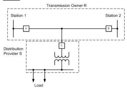
In Figure 4 above, the Interconnected Element between the Transmission Owner and the Distribution Provider is the transmission line or tap between the line and Breaker C.
