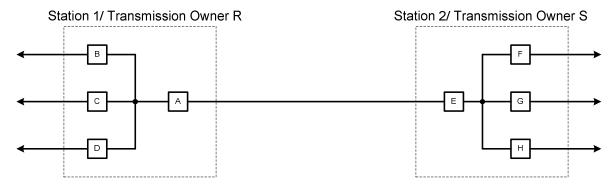
In Figure 1 above, the Interconnected Element between the Transmission Owners is the transmission line between Breakers A and E.
