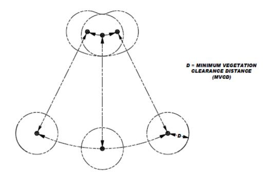
Cross-Section View of a Single Conductor At a Given Point Along The Span Showing Six Possible Conductor Positions Due to Movement Resulting From Thermal and Mechanical Loading For Consideration in Developing a Maintenance Approach
