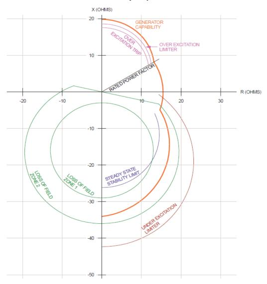
Section G Attachment 3 - Example of Capabilities, Limiters, and Protection on an Inverse Time Characteristic Plot
