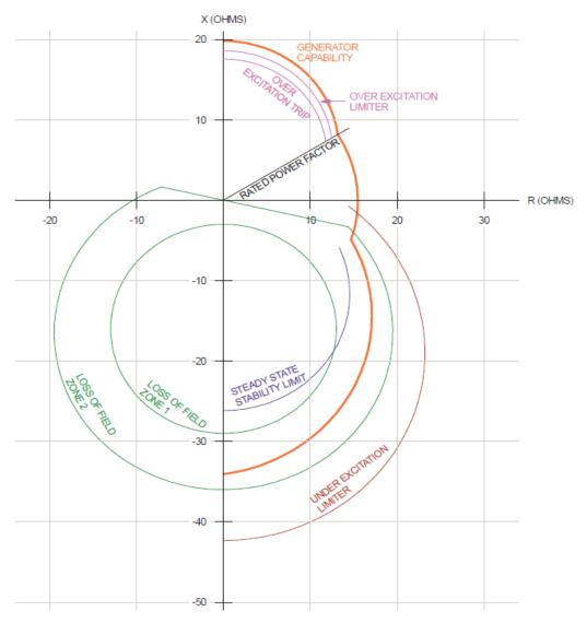
Attachment 3 - Example of Capabilities, Limiters, and Protection on an Inverse Time Characteristic Plot
