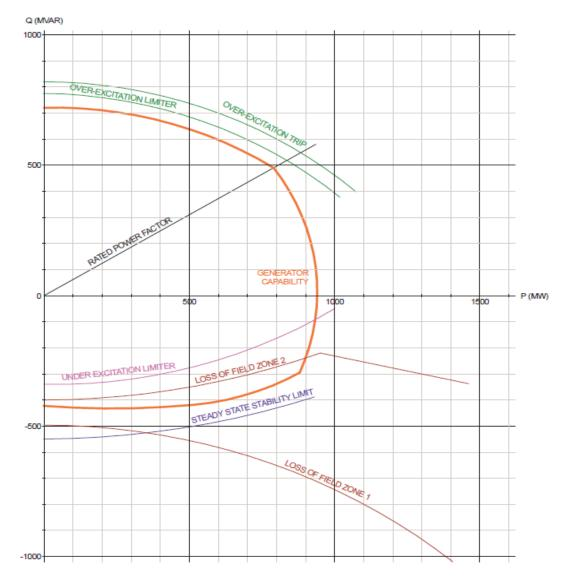
Attachment 2 – Example of Capabilities, Limiters, and Protection on an R-X Diagram at nominal voltage and frequency
