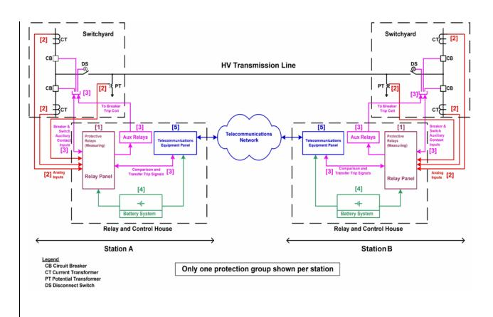
For information on numbered components, see Figure 1 & 2 Legend - Components of Protection Systems
