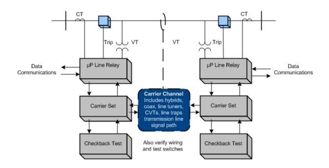
In this example (Figure A1), verification takes advantage of the self-monitoring features of microprocessor multifunction line relays at each end of the line. For each of the line relays themselves, the example assumes that the user has the following arrangements in place:
