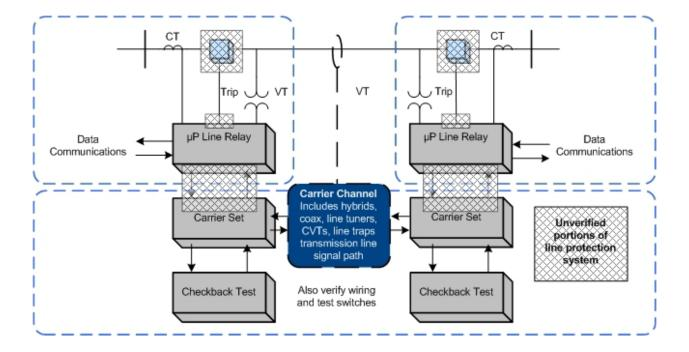
The dotted boxes of Figure A-2 show the sections of verification defined by the monitoring and verification practices just listed. These sections are not completely overlapping, and the shaded regions show elements that are not verified:
