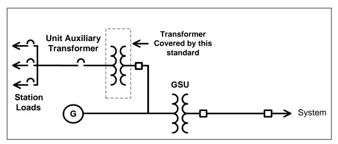
Figure-2 – Typical Auxiliary Power System for Power Plants
