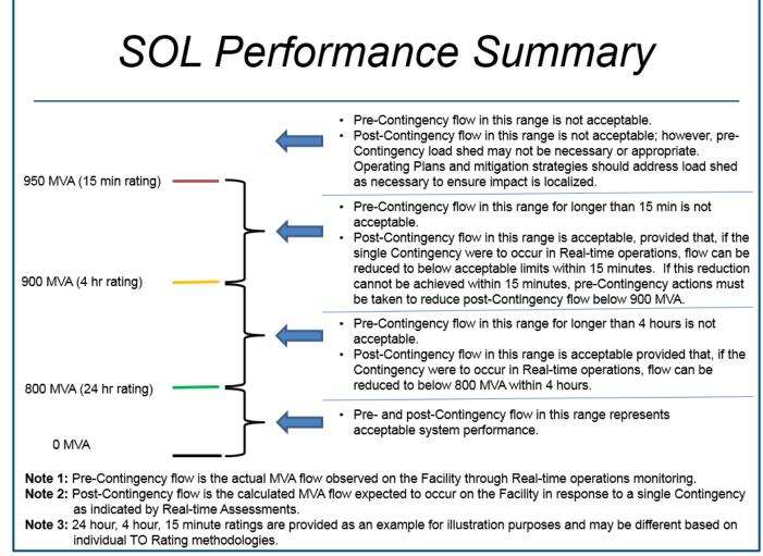
Figure 1. Facility Rating System Operating Limit Performance Summary
