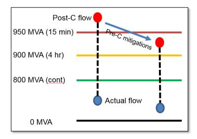
Figure 3. Example 2 Scenario – Unacceptable Post-Contingency State
