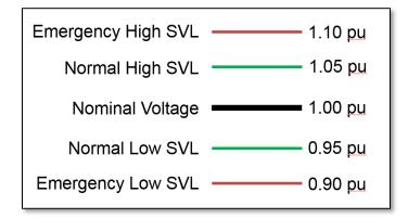
Figure 6. Example of a System Voltage Limit Set
