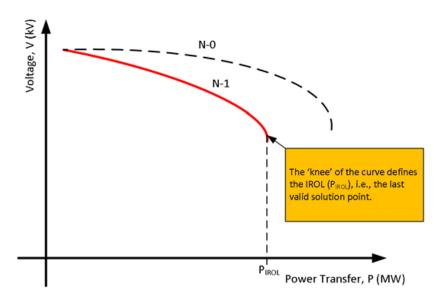
Figure 8. Voltage Stability System Operating Limit Performance Summary
