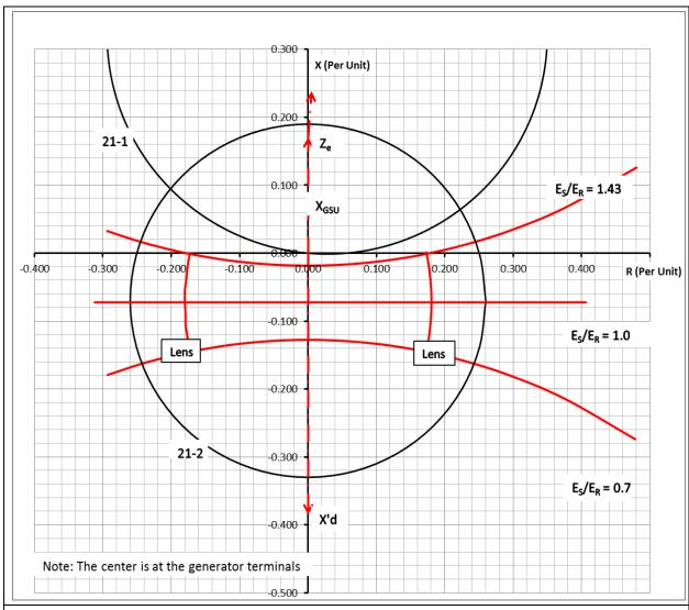
Figure 19: Swing impedance graph for impedance relays at a generating facility.
