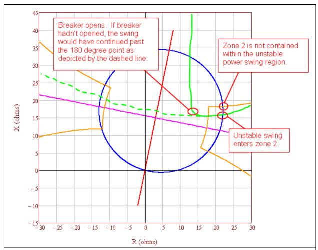
**Figure 24:** In this case, the Zone 2 element on circuit breakers 1, 2, 3, and 4 did not meet the PRC-026-12 — Attachment B criteria (this figure depicts the power swing as seen by relays on breakers 3 and 4).
