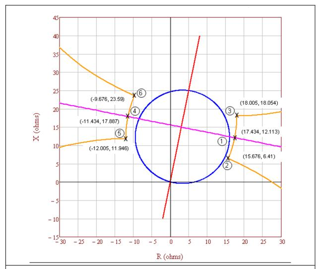
**Figure 4:** The defining unstable power swing region points where the lens shape intersects the lower and upper loss-of-synchronism circle shapes and where the lens intersects the equal EMF (electromotive force) power swing.
