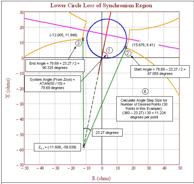
**Figure 15c:** Lower circle loss-of-synchronism region showing the steps to calculate the start angle, end angle, and the angle step size for the desired number of calculated points. 1) Calculate the system angle. 2) Calculate the start angle. 3) Calculate the end angle. 4) Calculate the angle step size for the desired number of points.
