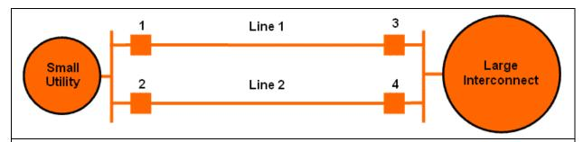
**Figure 23:** A simple electrical system where two lines tie a small utility to a much larger interconnection.
