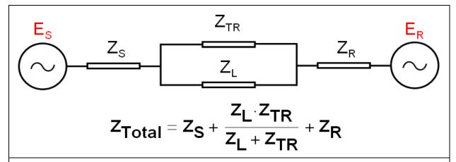
**Figure 6:** Reduced two bus system with sending-end source impedance  $Z_S$ , receiving-end source impedance  $Z_R$ , line impedance  $Z_L$ , and parallel transfer impedance  $Z_{TR}$ .
