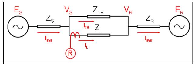
**Figure 13:** The infeed diagram shows the impedance in front of the relay R with the parallel transfer impedance included. As the parallel transfer impedance approaches infinity, the impedances seen by the relay R in the forward direction becomes  $Z_L + Z_R$ .
