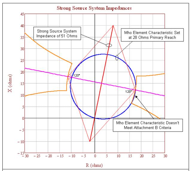
**Figure 8:** A strong-source system with a line impedance of  $Z_L = 20.4$  ohms (i.e., the thicker red line). This mho element characteristic (i.e., the blue circle) does not meet the PRC-026-1-2 – Attachment B, Criterion A because it is not completely contained within the unstable power swing region (i.e., the orange characteristic).
