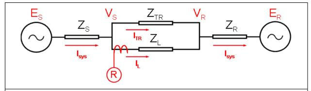
Figure 3: System impedances as seen by Relay R (voltage connections are not shown).
