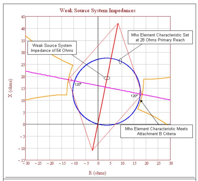
**Figure 9:** A weak-source system with a line impedance of  $Z_L = 20.4$  ohms (i.e., the thicker red line). This mho element characteristic (i.e., the blue circle) meets the PRC-026-1-2 – Attachment B, Criterion A because it is completely contained within the unstable power swing region (i.e., the orange characteristic).
