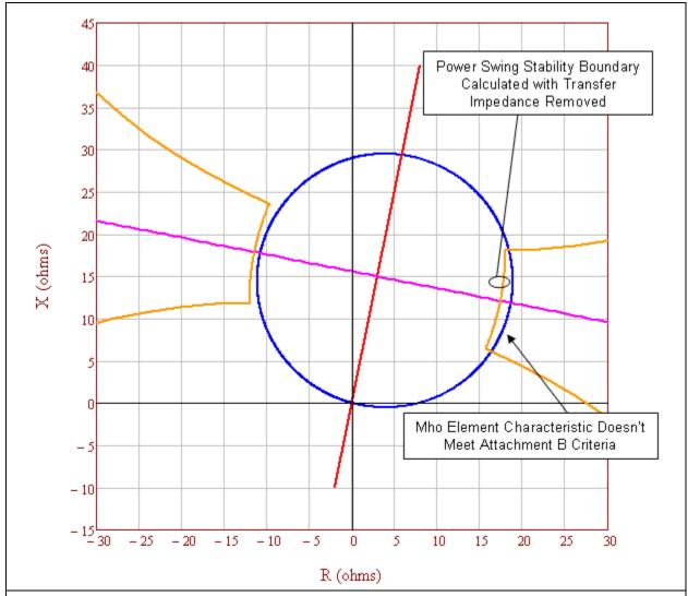
**Figure 10:** This is an example of an unstable power swing region (i.e., the orange characteristic) with the parallel transfer impedance removed. This relay mho element characteristic (i.e., the blue circle) does not meet PRC-026-1-2 — Attachment B, Criterion A because it is not completely contained within the unstable power swing region.
