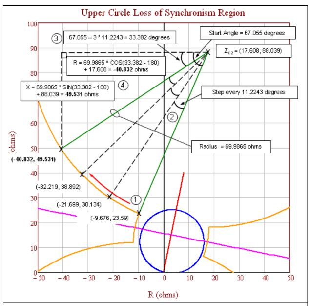
**Figure 15h:** Upper circle loss-of-synchronism region showing the final steps to calculate the coordinates of the points on the circle. 1) Start at the intersection with the lens shape and proceed in a clockwise direction. 2) Advance the step angle for each point. 3) Calculate the new angle after step advancement. 4) Calculate the R-X coordinates.
