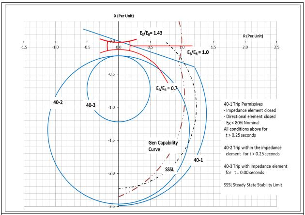
**Figure 20:** Typical R-X graph for loss-of-field relays with a portion of the unstable power swing region defined by PRC-026-<u>1-2</u> Attachment B, Criterion A.
