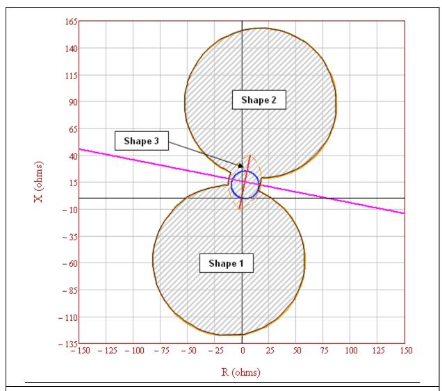
**Figure 2:** Full graphic of the unstable power swing region formed by the union of the three shapes in the impedance (R-X) plane: Shape 1) Lower loss-of-synchronism circle, Shape 2) Upper loss-of-synchronism circle, and Shape 3) Lens. The mho element characteristic is completely contained within the unstable power swing region, therefore it meets PRC-26-1 – Attachment B, Criterion A, No.1.
