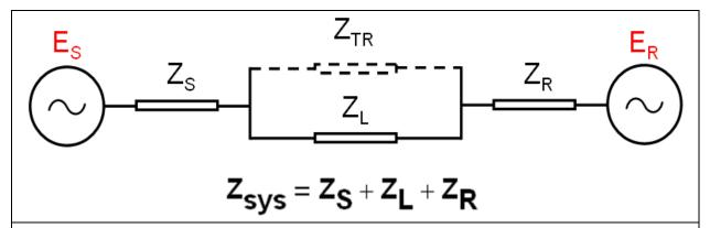
**Figure 7:** Reduced two bus system with sending-end source impedance  $Z_S$ , receiving-end source impedance  $Z_R$ , and line impedance  $Z_L$  with the parallel transfer impedance  $Z_{TR}$  removed.
