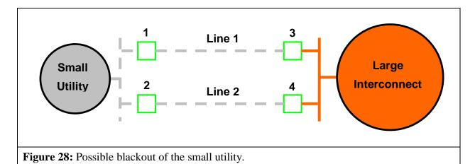
If the relays that tripped in response to the previous unstable power swing condition in Figure 24 were addressed under the Requirements to meet PRC-026-12 - Attachment B criteria, the unnecessary tripping of the relays for the stable power swing shown in Figure 28 would have been averted, and the possible blackout of the small utility would have been avoided.
