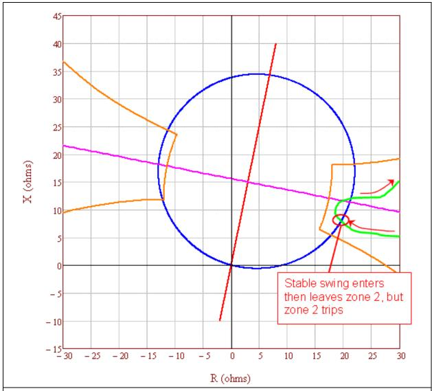
**Figure 27:** Relays on circuit breakers 2 and 4 were not addressed to meet the PRC 026 1 PRC 026-2 — Attachment B criteria following the previous unstable power swing event.
