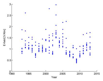
Figure I-3: Scatter Plot of Ten Largest Geoelectric Fields per Year Data source: IMAGE magnetometer chain from 1993-2013
