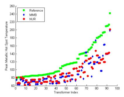
Figure I-7: Calculated <u>peak metallic hot spot temperaturePeak Metallic Hot Spot</u> <u>Temperature</u> for <u>all transformersAll Transformers</u> in a <u>test systemTest System</u> with a <u>temperature increaseTemperature Increase</u> of <u>more thanMore Than</u> 20°C for <u>dD</u>ifferent GMD <u>events scaledEvents Scaled</u> to the <u>same peak geoelectric fieldSame</u> <u>Peak Geoelectric Field</u>
