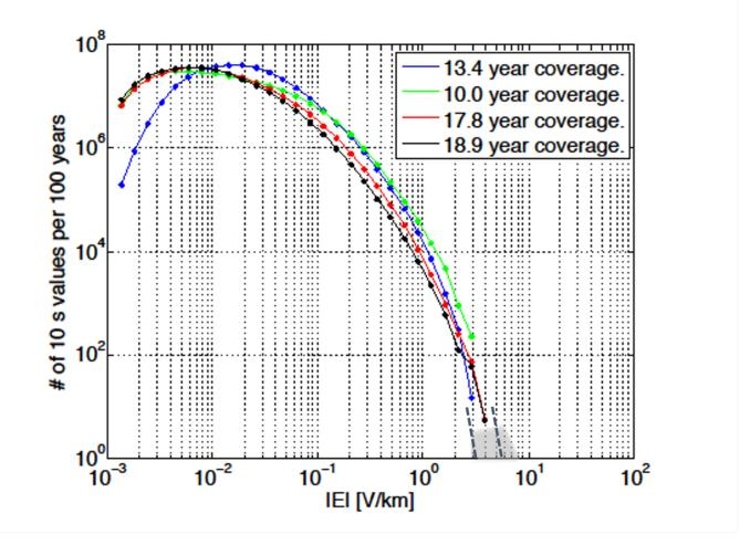
**Figure I-2: Statistical eQccurrence of** spatially averaged geoelectric field amplitudesSpatially Averaged Geoelectric Field Amplitudes. Four curves with dots correspond to different station groups and the gray area shows a visual extrapolation to 1-in-100 year amplitudes. Dashed lines represent the values predicted with extreme value analysis. The legend shows the data coverage for each station group used in computing the averaged geoelectric field amplitudes.
