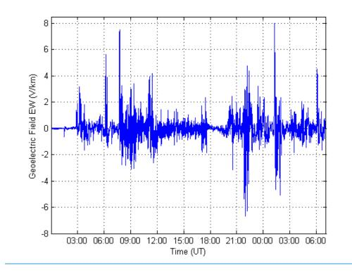
Figure 2: Benchmark Geoelectric Field Waveshape (E<sub>E</sub> Eastward)
