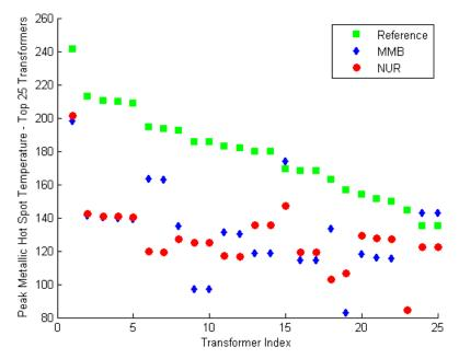
Figure I-8: Calculated <u>peak metallic hot spot temperaturePeak Metallic Hot Spot</u> <u>Temperature</u> for the <u>t</u>op 25 <u>t</u>ransformers in a <u>test systemTest System</u> for <u>dD</u>ifferent GMD <u>events scaledEvents Scaled</u> to the <u>same peak geoelectric fieldSame</u> <u>Peak Geoelectric Field</u>
