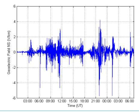
Figure 3: Benchmark Geoelectric Field Waveshape ( $E_N$  Northward)
