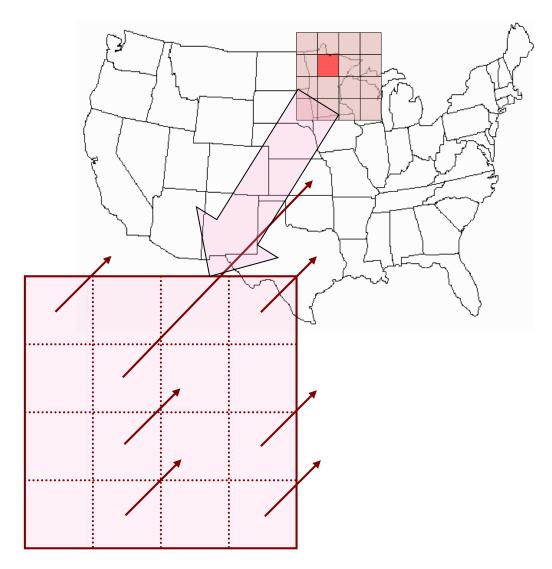
Figure I-1: Illustration of the spatial scaleSpatial Scale between localized enhancementsLocalized Enhancements and larger spatial scale amplitudesLarger Spatial Scale Amplitudes of geoelectric field observedGeoelectric Field Observed during a strong geomagnetic storm. Strong Geomagnetic Storm. In this illustration, the red square illustrates a spatially localized field enhancement.
