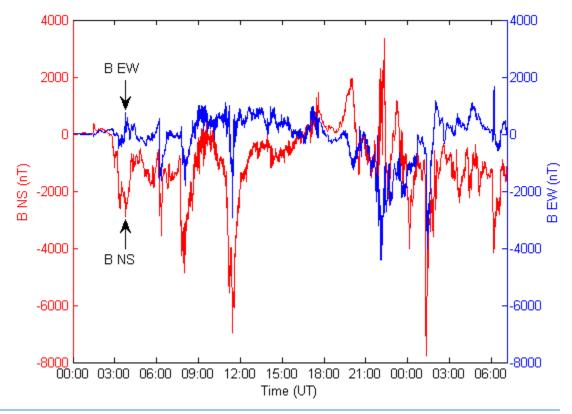
Figure 1: Benchmark Geomagnetic Field Waveshape Red Bn (Northward), Blue Be (Eastward)
