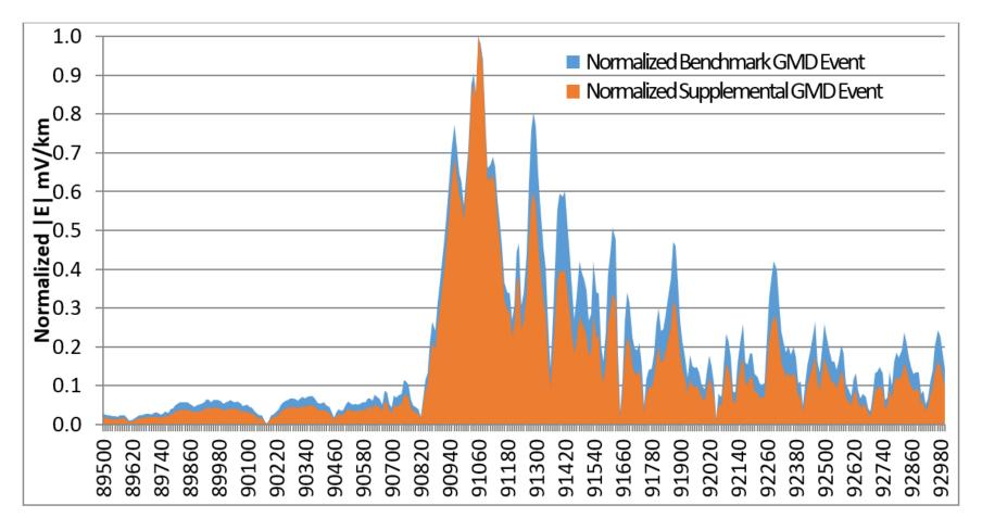
In other words, if the peak transformer GIC screening threshold were 75 A/phase for both events, the transformer suffering a supplemental GMD event would experience less overall heating; the aggregated effects of the Supplemental geoelectric field "intensity" is not sustained. Thus, the screening threshold for supplemental GMD event transformer GIC is established at a slightly higher, but conservative, 85A/phase.
