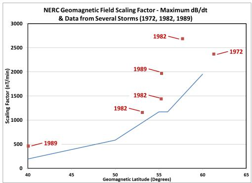
Figure 2 – NERC 100 Year Storm Reference Profile and Observations od dB/dt in 1972, 1982 and 1989 Storms that exceed the NERC Reference Profile
