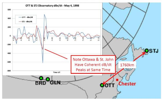
Figure 3. Magnetometer Readings Over Time from Ottawa and St. John Observatories
