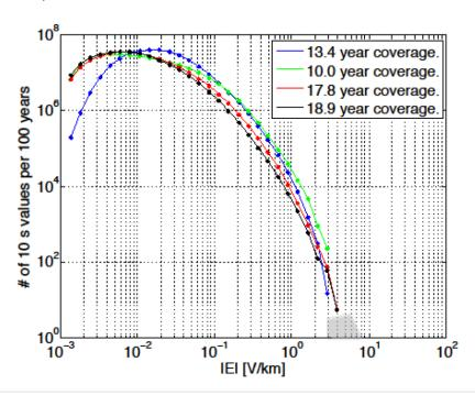
**Figure I-2: Statistical Occurrence of Spatially Averaged Geoelectric Field Amplitudes.** Four curves with dots correspond to different station groups and the gray area shows a visual extrapolation to 1-in-100 year amplitudes. The legend shows the data coverage for each station group used in computing the averaged geoelectric field amplitudes.
