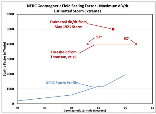
Figure 6 – Scientific Estimates of Extreme Geomagnetic Storm Thresholds compared to Propose3d NERC Draft Standard
