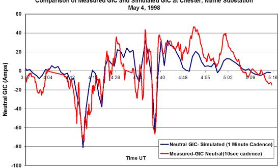
Comparison of Measured GIC and Simulated GIC at Chester, Maine Substation
