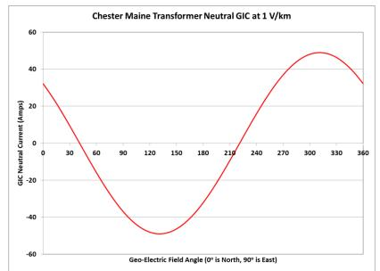
Figure 7 - GIC flow at Chester transformer neutral for 1 V/km geo-electric field at various orientation angles.
