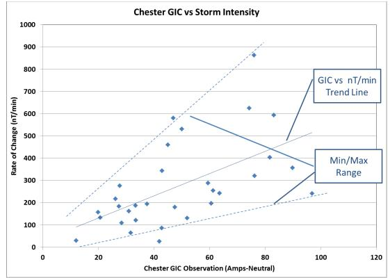
Figure 4 – GIC versus Storm Intensity (nT/min) from multiple observed GIC storm events at Chester Transformer, in this case the GIC timing is extremely coarse.
