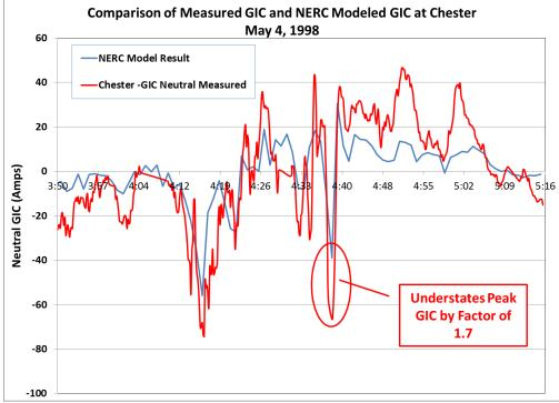
Figure 18 - Comparison of NERC model GIC to observed GIC at Chester.
