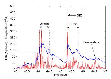
Figure 3: Sample Tie Plate Temperature Calculation
