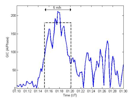
Figure 15: Close-up of GIC(t) and a Five Minute 180 A/phase GIC Pulse at Full Load
