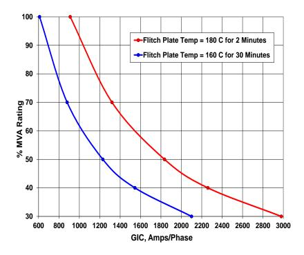
Figure 2: Sample GIC Manufacturer Capability Curve of a Large Single-Phase Transformer Design using the Flitch Plate Temperature Criteria [3]
