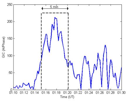
Figure 16: Close-up of GIC(t) and a 5 Minute 225 A/phase GIC Pulse Assuming 75% Load
