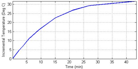
Figure 7: Thermal Step Response to a 16.67 Amperes per Phase dc Step Metallic hot spot heating.
