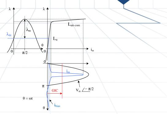
Figure 1: Mapping Magnetization Current to Flux through Core Excitation Characteristics
