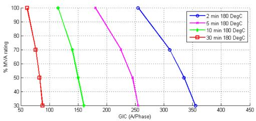
Figure 12: Capability Curve of a Transformer Based on the Thermal Response Shown in Figures 8 and 9.
