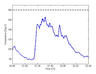
Figure 11: Close-up of Metallic Hot Spot Temperature Assuming a 75% Load (Oil temperature of 64.5°C)
