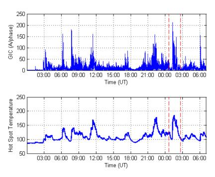
Figure 9: Magnitude of GIC(t) and Metallic Hot Spot Temperature  $\theta$ (t) Assuming Full Load Oil Temperature of 85.3°C (40°C ambient). Dashed lines approximately show the close-up area for subsequent Figures.
