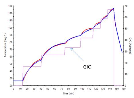
Figure 9: Comparison of measured temperatures (red trace) and simulation results (blue trace). Injected current is represented by the magenta trace.
