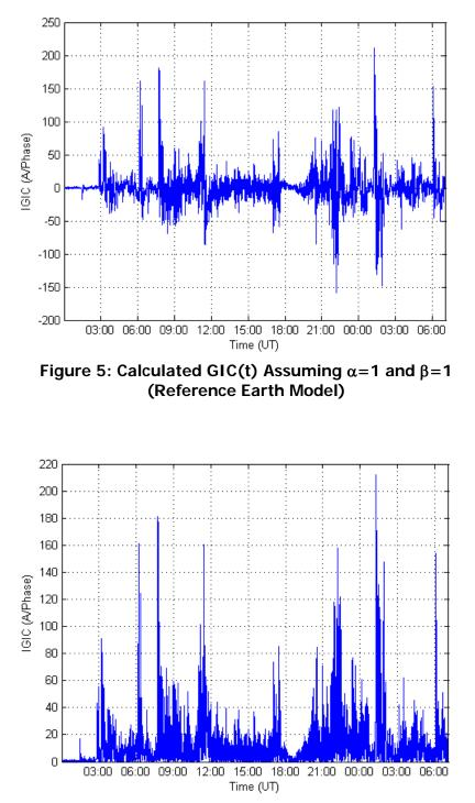
Figure 6: Calculated Magnitude of GIC(t) Assuming  $\alpha$ =1 and  $\beta$ =1 (Reference Earth Model)
