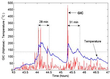
Figure 3: Sample Tie Plate Temperature Calculation
