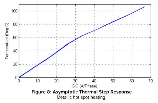
The step response in **Figure 7** was obtained from the first GIC step of the tests carried out in [6]. The asymptotic thermal response in **Figure 8** was obtained from the final or near-final temperature values after each subsequent GIC step. **Figure 9** shows a comparison between measured temperatures and the calculated temperatures using the thermal response model used in the rest of this discussion.
