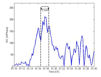
Figure 15: Close-up of GIC(t) and a 2 minute 255 A/phase GIC pulse at full load
