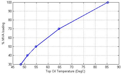
Figure 14: Simplified Loading Curve Assuming 40°C Ambient Temperature.
