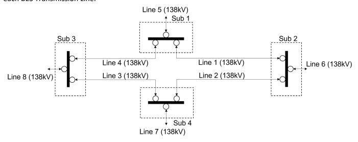
Note: Substation equipment (e.g., transformers) is not shown for simplicity. Circles represent fault interrupting devices.
