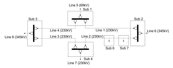
Note: Substation equipment (e.g., transformers) is not shown for simplicity. Circles represent fault interrupting devices.
