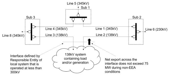
Note: Substation equipment (e.g., transformers) is not shown for simplicity. Circles represent fault interrupting devices.
