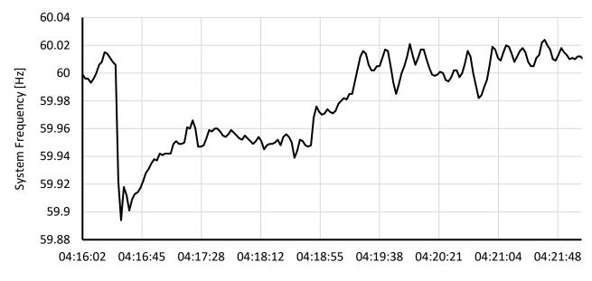
Figure I.6: System Frequency Response for First Fault Event
