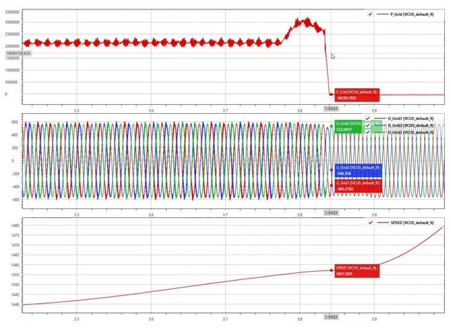
Figure 1.9: Turbine High Speed Data Capturing Turbine Tripping for Different Event
