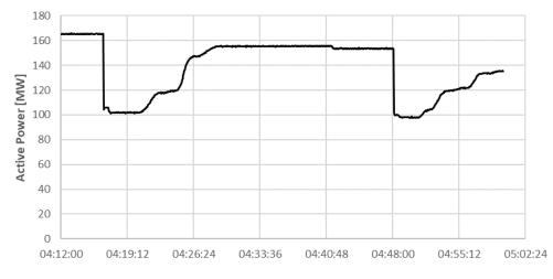
Figure A.10: Plant Active Power Output
