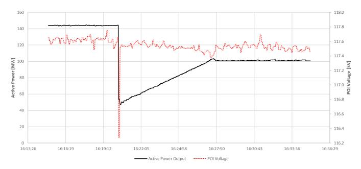
Figure B.1: Overall Wind Plant Response to BPS Fault
