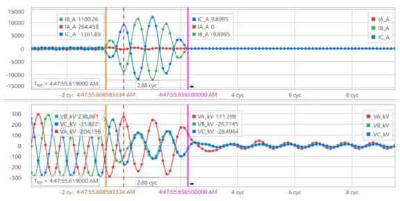
Figure I.3: B-C Fault on 345 kV Transmission Circuit [Source: Oncor]
