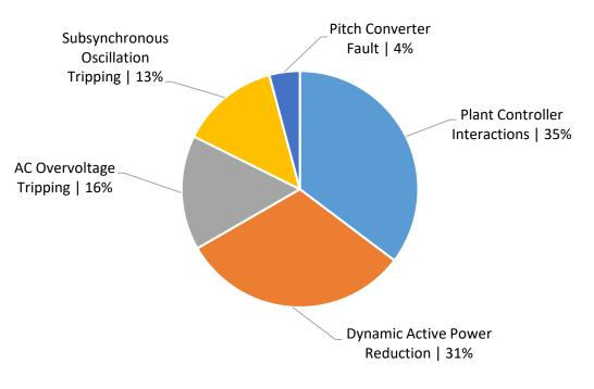
Figure 1.2: Causes of Wind Plant Reduction for Fault 2
