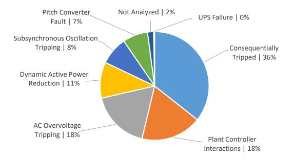
Figure 1.1: Causes of Wind Plant Reduction for Fault 1
