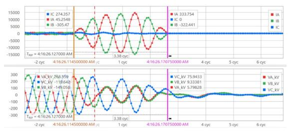
Figure I.2: A–B Fault on Generator Tie Line [Source: Oncor]
