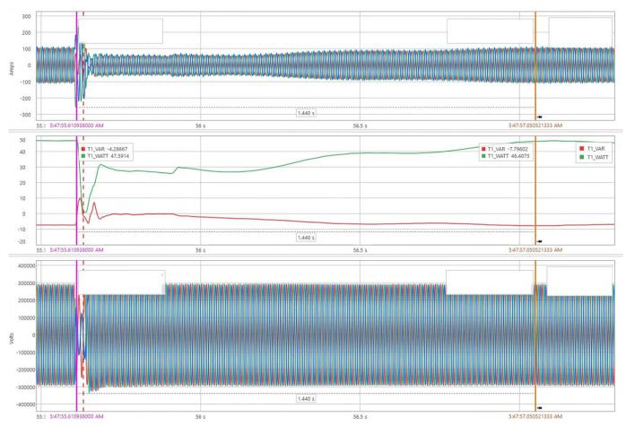
Figure 1.5: Dynamic Response of Plant to Second Fault
