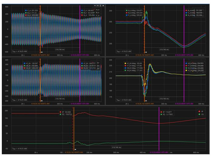
Figure A.2: Wind Plant Dynamic Response during Fault 1
