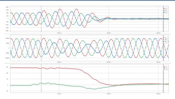
Figure B.2: High Speed Oscillography Data at POI Showing Plant Response to Fault
