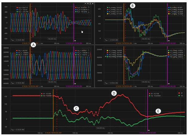
Figure 1.3: Abnormal Dynamic Response of Wind Power Plant
