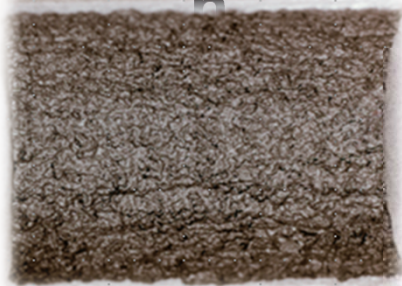
Pitting (Electrical Phenomena)
